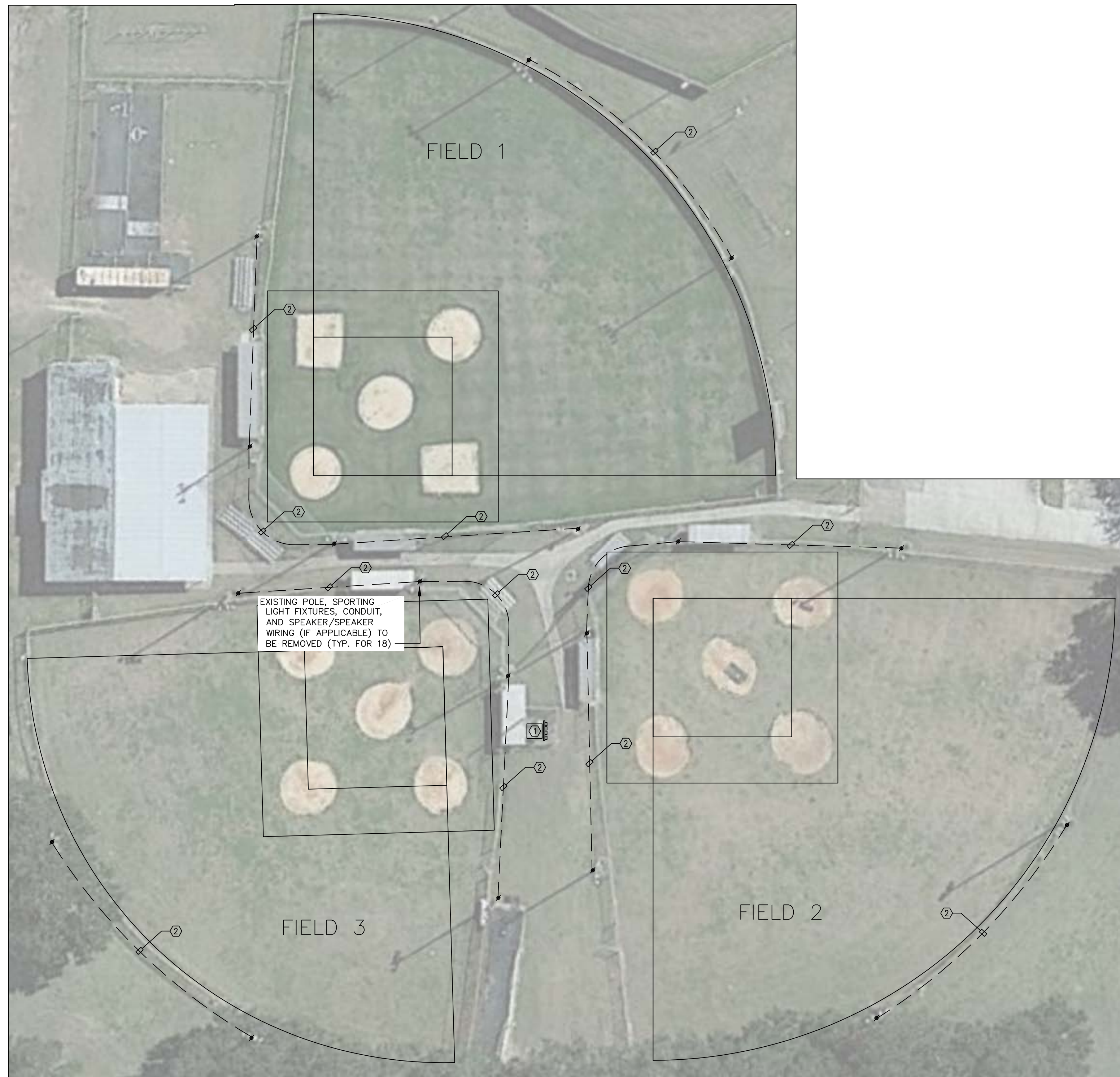
NORTH 1 ELECTRICAL DEMOLITION PLAN SCALE = 1" = 30'-0"
